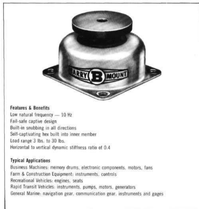
Figure 13 — Captive Elastomeric Mount.
