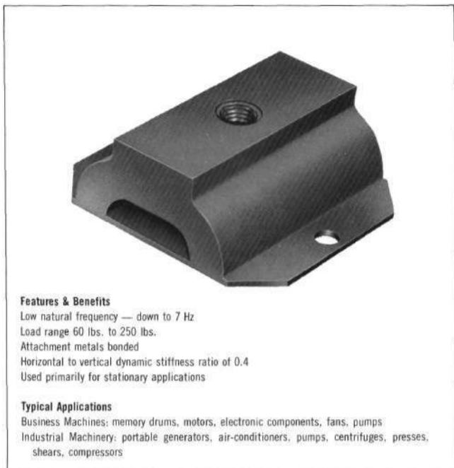
Figure 12 — General Purpose Elastomeric Compression Mount.
